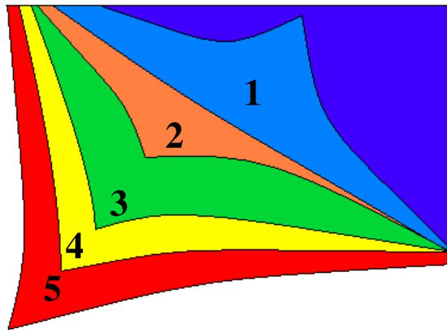
1. Top Lacquer 2. Print Design 3. Top Ply of Aqualux™ Film 4. Bottom Ply of Aqualux™ Film 5. Bottom Lacquer
